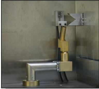
Inner dia. of tube is 11mm, tube and vertical line as 25° .
